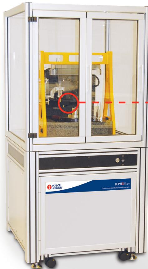
LuphoScan is an interferometric, scanning metrology system based on MWLI<sup>®</sup> technology (multi-wavelength interferometry), designed to perform fast, ultra precision non-contact 3D form measurement.
