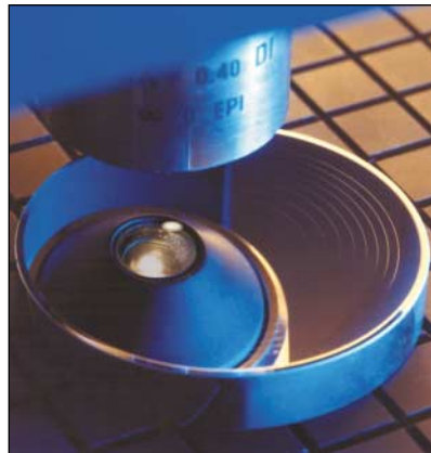
micro roughness, waviness, feed rate and depth of cut on diamond turned surfaces can be evaluated
