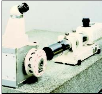
TB80 and autocollimator used to check polygons
