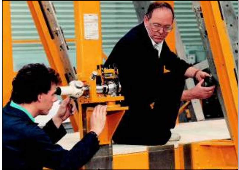
Checking Aircraft jigs with Micro Alignment Telescope
