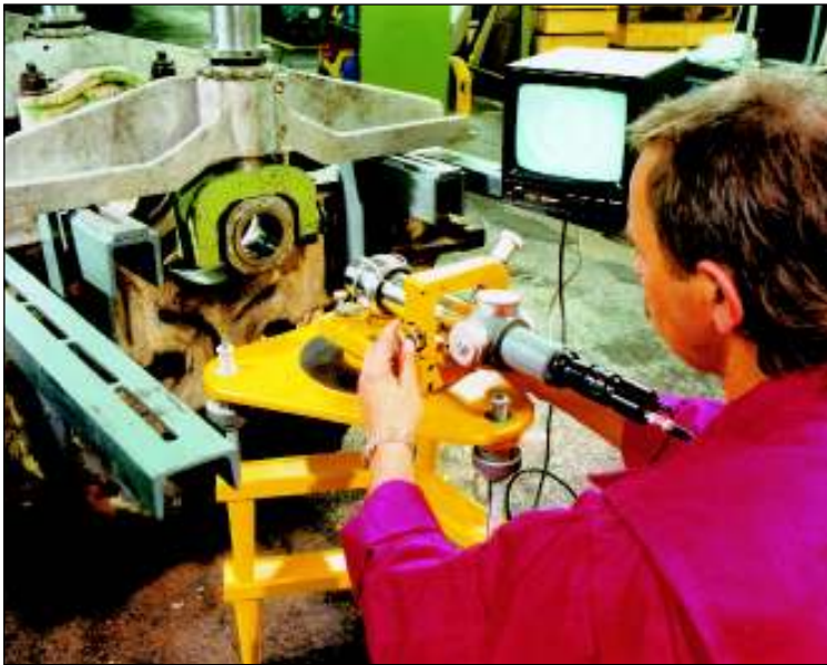
Aligning diesel engine bearings using CCTV and Micro Alignment Telescope
