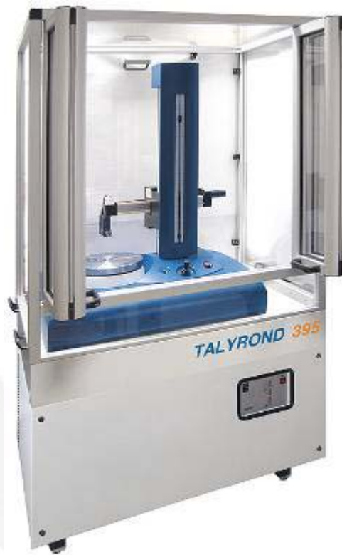
Talyrond 395 Automatic Roundness and Cylindricity
